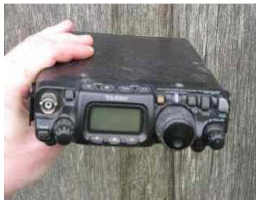
Yaesu was the first mainstream manufacturer to bring out a very small portable multiband transceiver with the FT-817 (pictured above) weighing about a kilogram. Launched in 2001, it featured 160 to 70 centimetre multimode coverage and a 5 watt output power. Icom responded with the bulkier and lower coverage 10-watt IC703.
